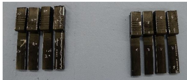
Figure 7: The tensile bars from both sides of the electrofusion joint
